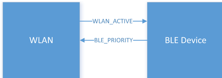
Figure 18-1 BLE Two-Wire Signaling
